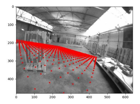
A frame from sequence indoor forward 5 with the virtual points projected according to the ground truth. The points should be coplanar with the ground but visibly are not. See also the video below.
