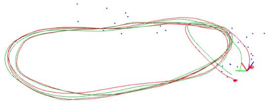
Fig. 1. Ground truth (green) and estimated (red) trajectory on the *indoor\_45\_4* sequence using the proposed method.
